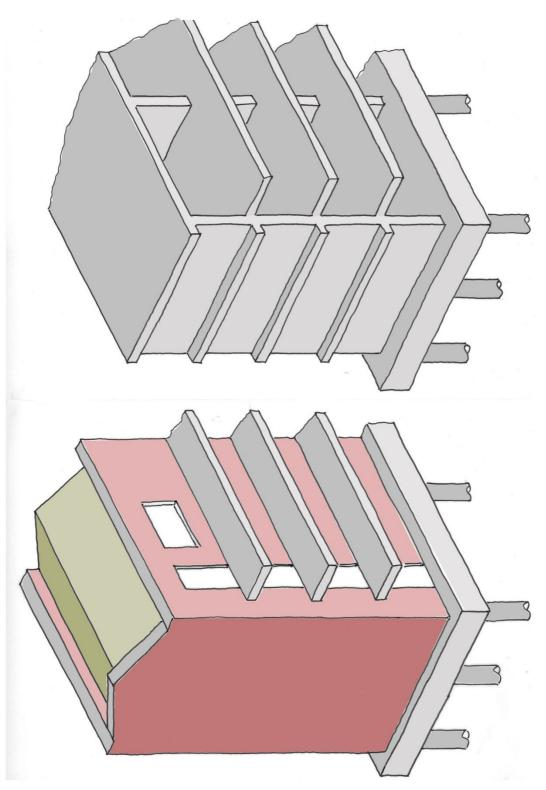
The brickwork is not part of the primary structure
