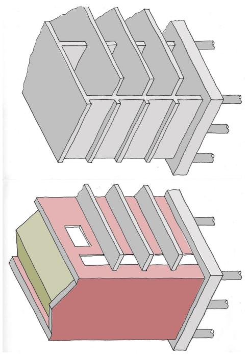
The brickwork can be removed from the stair cores and gable ends without compromising stability or weather-tightness
